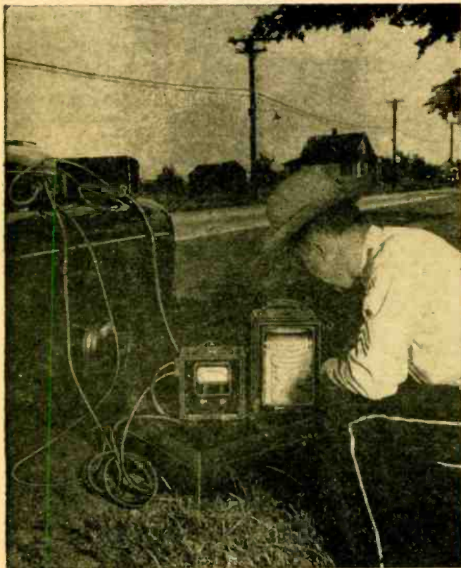
The radar transmitter-receiver is on the car's trunk compartment.
